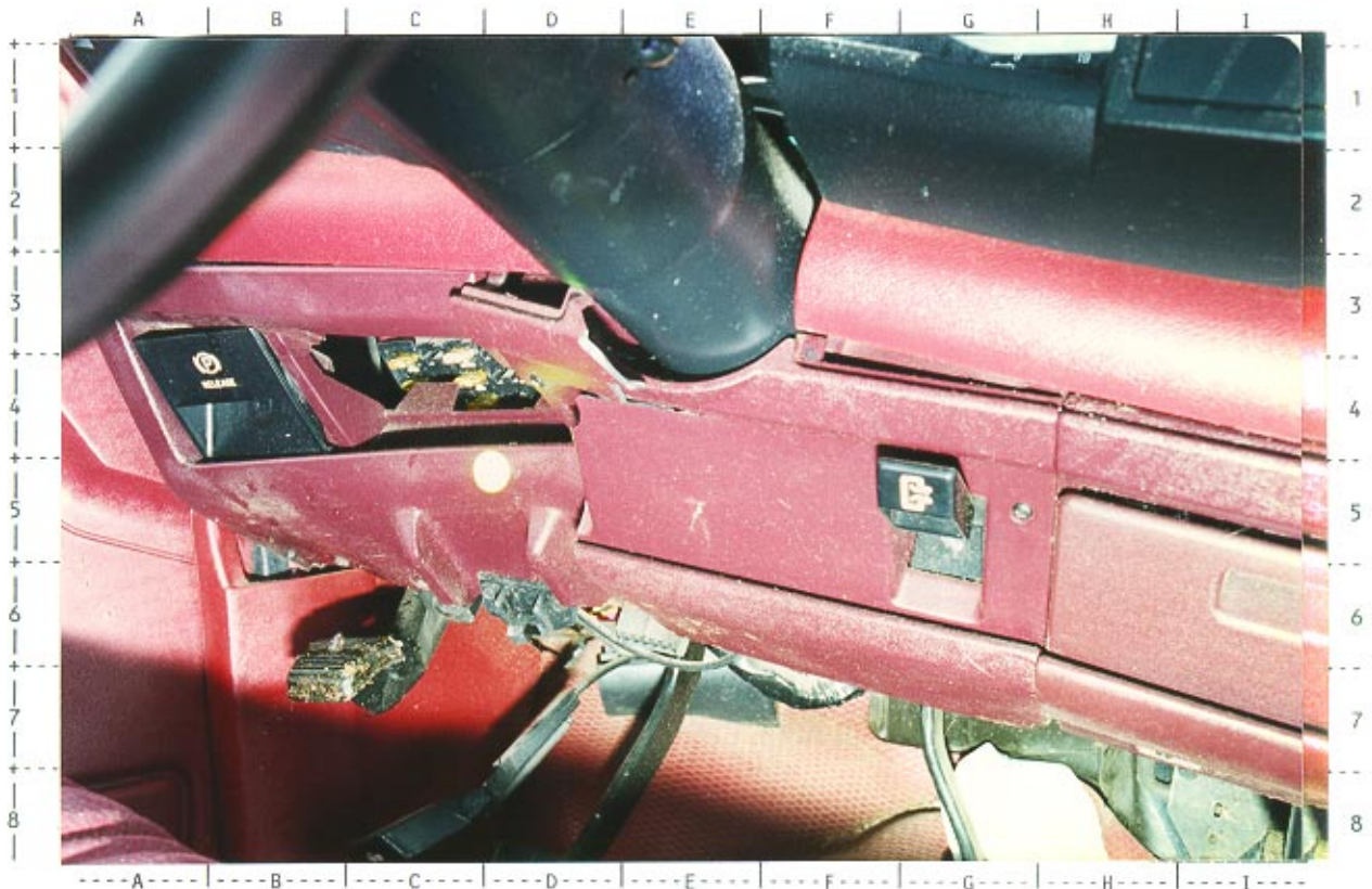
# 83 -- Close-up of left knee contact to 1988 Chevrolet pickup's left lower dash area; NOTE: entrapment occurred in toe pan area
